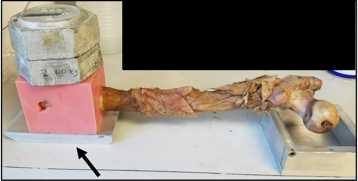
Figure 3-3 Potted femur positioned for head cast creation. Metal plates were utilized to raise or lower the specimen.
