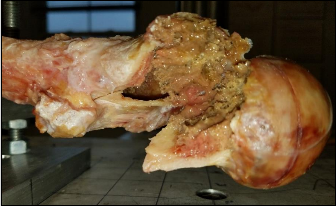
Figure 5-5 Fracture location in the specimen with the lateral lesion as viewed from the medial side. The fracture line ran subcapitally and to the lesser trochanter, nearly removing the entire femoral head.
